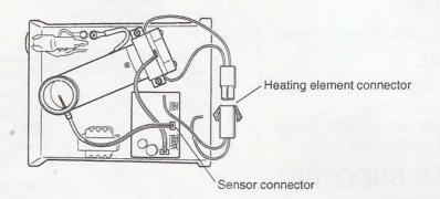
Heating element resistance measurement
