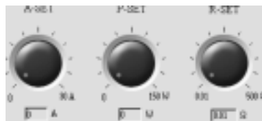
Fig.2-4 (1) Setup the Current Value, the Power Value and the Resistance Value Using Rotary
