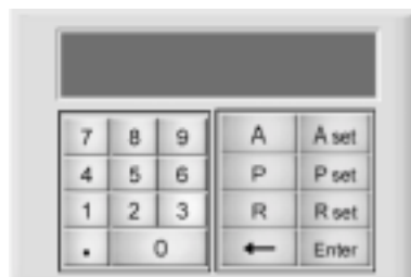
Fig.3-4(2) Setup the Current, Power and Resistance Using the Keyboard
